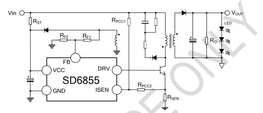
2) SD6856 adopts an external driving MOSFET suitable for 5~7W output power. Output 7W application is shown below: output 25V/300mA;
