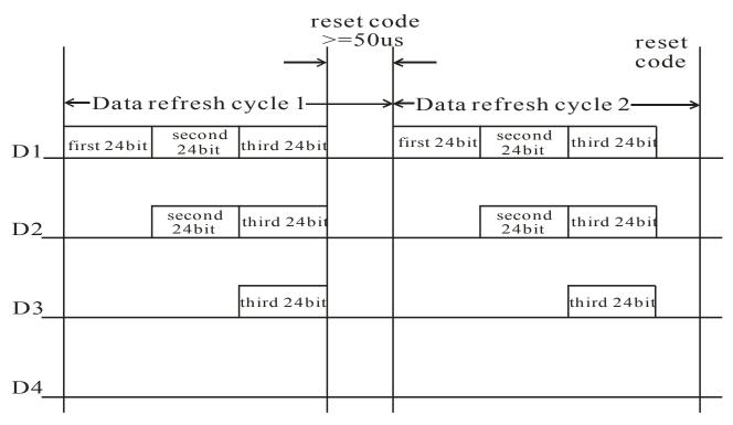
Note: The data of D1 is send by MCU, and D2, D3, D4 through pixel internal reshaping amplification to transmit.
