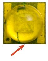
It is not required to use a solder footprint for the thermal pad that is larger than the XLamp XT Family LED itself. In testing, Cree LED has found such a solder pad to have insignificant impact on the resulting T<sub>a</sub> measurement.
