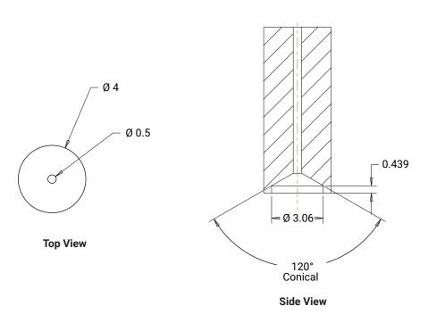
The following diagram shows an example of a pick & place tool to remove XLamp XP-E2, XP-G2 and XP-G3 LEDs from the factory tape & reel packaging. The nozzle is implemented in urethane.
