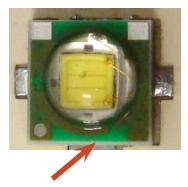
It is not required to use a solder footprint for the thermal pad that is larger than the XLamp XP Family LED itself. In testing, Cree LED has found such a solder pad to have insignificant impact on the resulting  $T_{a}$  measurement.
